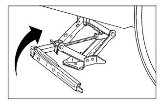
5. Raise the vehicle by turning the jack handle clockwise. Raise the vehicle far enough off the ground so there is enough room for the road tire to be removed.
